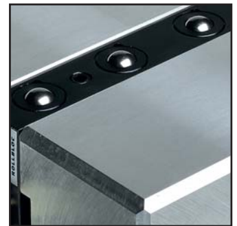
The press table is equipped with ROLLBLOC die lifters when using Rollbloc interchangeable subplate technology
