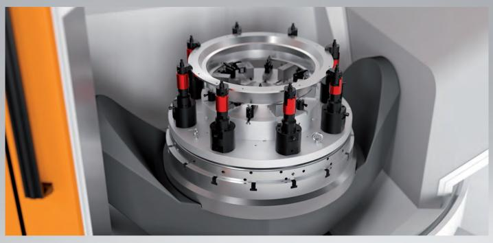
In the milling and turning process, cables are often in the way due to the changing positioning of the rotary table or do not offer the necessary flexibility in order to follow the movements of the fixture. By using the AMF Wireless sensoring systems, the workpiece support can be queried easily and with process reliability and without laboriously laying cables.
