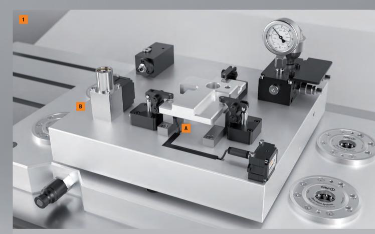
The hydraulic clamping fixture is provided with two queries. The workpiece location pad is queried via a microswitch **A** with a connected Sender-Unit. The wireless pressure switch **B** monitors the pressure of the clamping fixture hydraulic clamping circuit.
