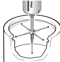
These stylus clusters provide you with multiple-tip probing of complex features and bores. Four or five ruby ball systems are mounted rigidly on a stainless steel center. Three standard sizes are offered – alternatively, you can create custom-made star styli using a 5-way stylus center and any of the genuine Renishaw stylus range.
