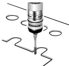
These are used for probing holes in thin sheet material. In addition, various threaded features can be probed and the centers of tapped holes located. Ball-ended cylinder styli allow full datuming and probing in X, Y and Z directions, thus allowing surface inspection to be performed.
