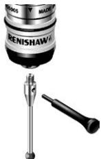
The S7 stylus tool is used for tightening styli and accessories when connecting to one another or directly into the probe. It is specifically designed to yield if excessive tightening force is applied, avoiding damage to the threads of stylus and probe.
