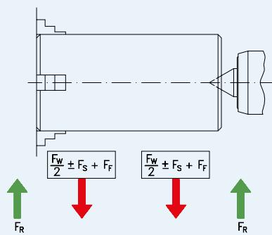
The formula is applicable when the workpiece weight FW is equally divided between headstock and tailstock. If the component has an irregular shape, the weight has to be split up correspondingly. The radial cutting force FS has to be either a positive or negative figure, depending on the direction of rotation. Any unbalance of the workpiece has to be allowed for with the centrifugal force FF.
