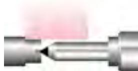
Short grinding length, wide grinding wheel, extended carbide centre
