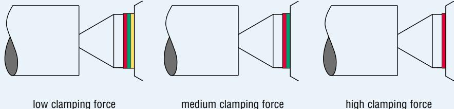
The yellow, green and red ranges of axial forces are permanently laser marked on the heads of the centre housings.
