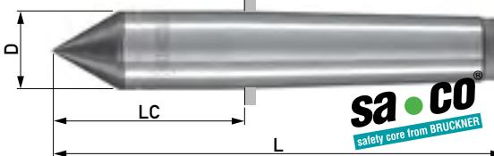
\* without safety core, carbide brazed in tapered seating
