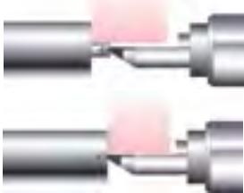
Small diameter or short grinding length or face grinding. Extended carbide half centre with extra small flat height
